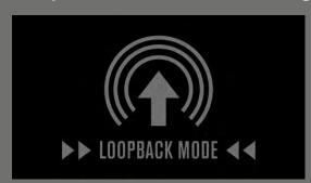
The Loopback function of the UR interfaces offers an easy way to stream performances live to the Internet. Often used by hosts of live online broadcasts, when the function is active, incoming audio signals to the UR (such as microphone, guitar or line source) are merged with the signal coming from audio playback software like Cubase or another DAW inside the computer. The merged signal will then be sent back to the computer for online streaming via your software of choice.
